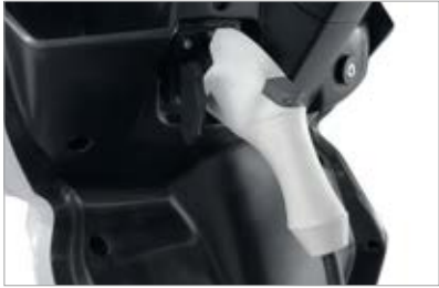
In addition to 200V outlet, J1772 socket enables charging with ordinary charger for automobiles.
