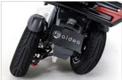
Right and left independent suspension rear suspension that enables stable running on rough roads and steps.
