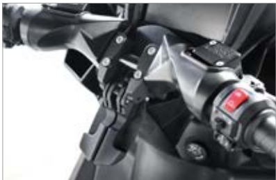
Roll lock lever to fix the vehicle vertically and parking lever to fix the vehicle in the front-rear direction.
