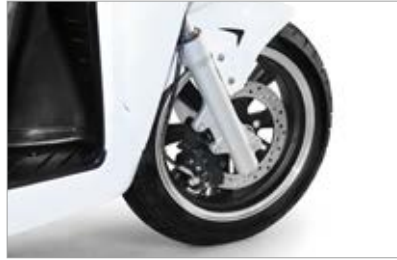
Combination brakes (front and rear disc brakes) that link the front and rear to provide stable braking force.
